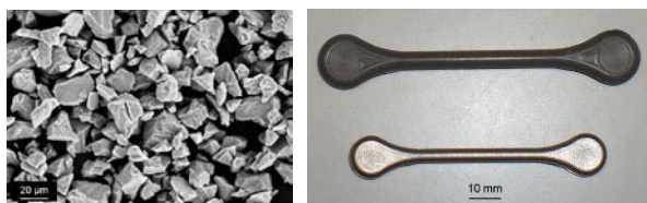
Fig. 1: Titanium hydride powders, injection moulded and sintered titanium parts
