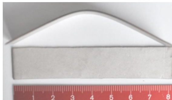
Figure 9. Tape cast porous titanium thin sheets before and after bending
