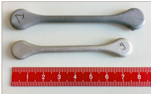
Fig. 4 Injection moulded and sintered MIM Ti-17Nb test specimens
