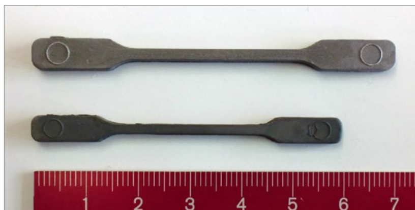
Fig. 5 MIM P558 austenitic stainless steel green (top) and sintered (bottom) specimens
