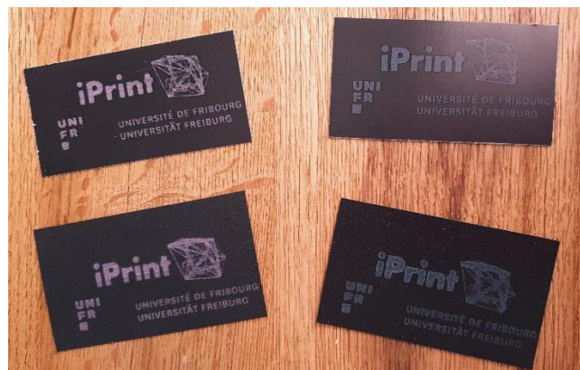
Figure 3. Photonic balls printed by means of inkjet technology. Left: Redish color. Right: Greenish color
