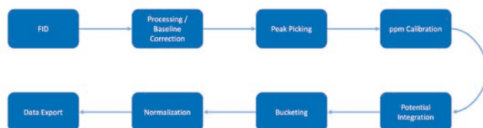
Fig. 9. Generic NMR workflow.
