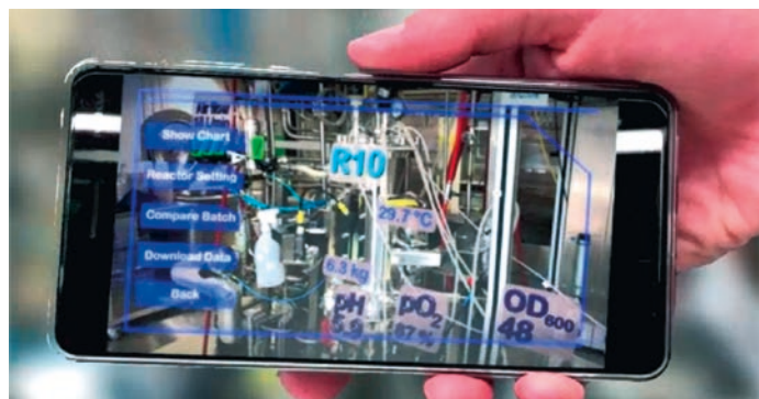
Fig. 8. Concept for AR visualization of bioprocess data on mobile devices. In context-sensitive displays, the most relevant key information is directly accessible.
