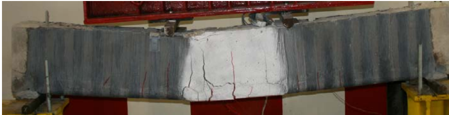
Figure 7: RC-COR1S2 beam after testing to failure.
