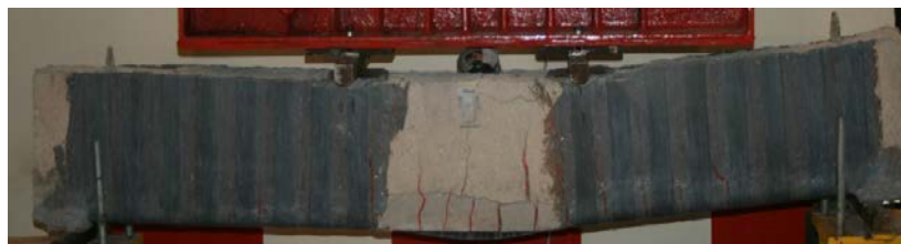
Figure 6: RC-COR1S1 beam after testing to failure.
