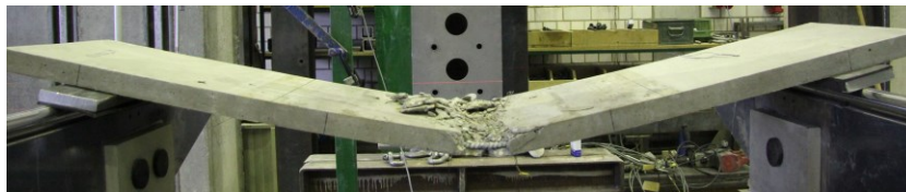
Figure 10. Post-heating bending. Typical failure mode of the panels.
