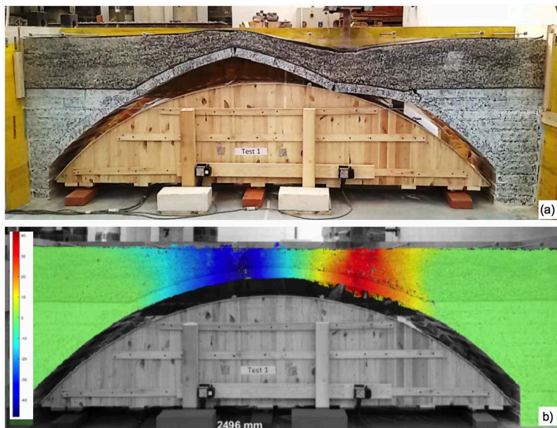
Figure 3. Laboratory tests on real-scale in-folio vaults retrofitted with Textile Reinforced Mortar: a) collapse configuration and b) analysis of the displacement field with Digital Image Correlation.
