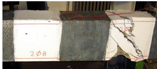
(ii) Wrapping with FRP strips
