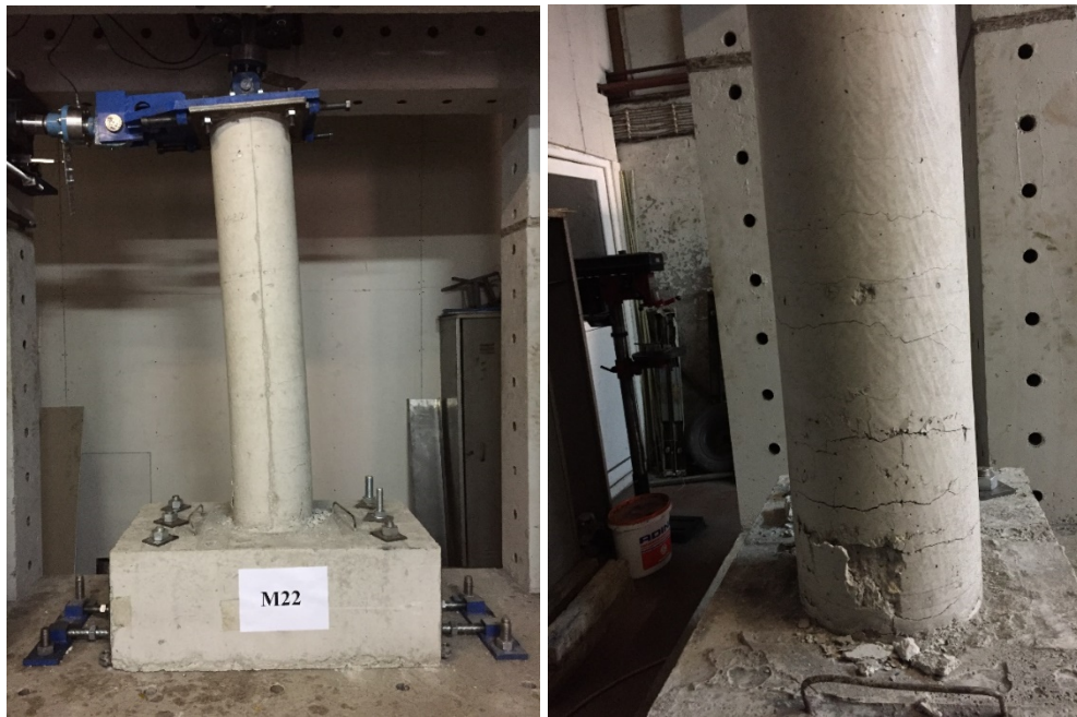
Figure 11 - Testing Frame and Testing of Columns
