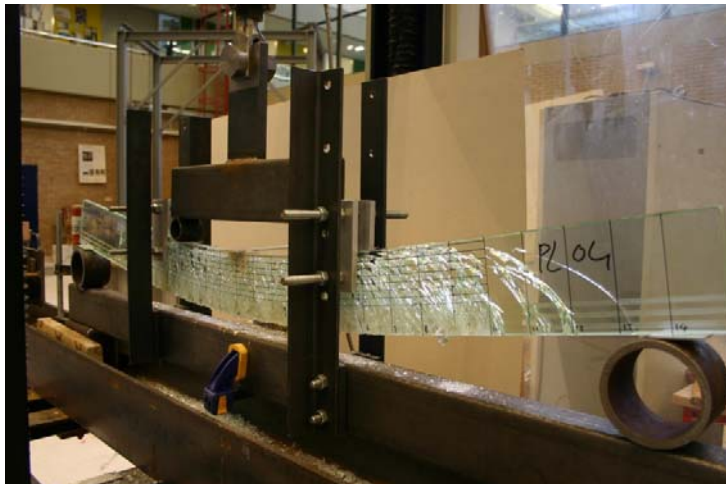
Figure 4: Composite glass beam with GFRP reinforcement during bending test. (Louter, 2011)
