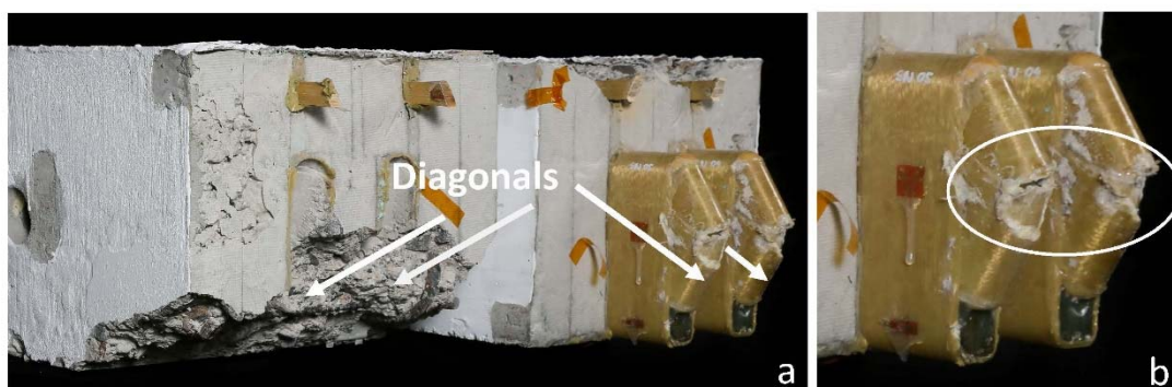
Figure 8. Failure mode of beam A200: a) bottom concrete spalling in interior (left) beam, b) wrinkling/crushing of AFRP hexagon diagonal.
