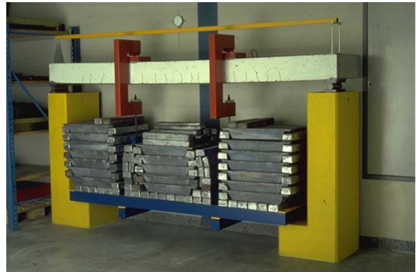
Reinforce concrete beam strengthenend with a steel plate glued with an epoxy. Long-term test since 1970.
