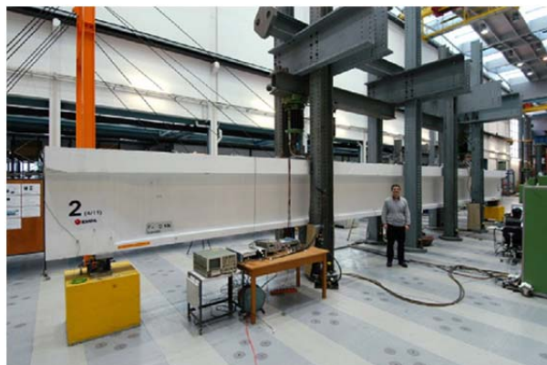
Figure 3: Bridge girder in the Empa laboratory and the force-deflection diagram of the experiments by Czaderski et al. [5] and [16] to show the feasibility of the gradient anchorage method.
