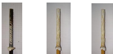
Figure 8: Typical failure modes observed after pull-out tests.
