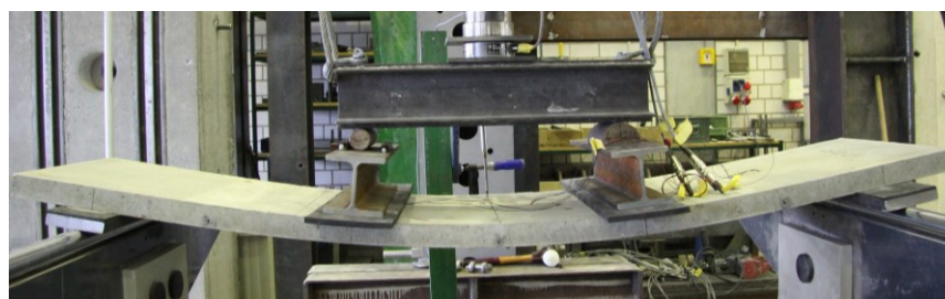
Figure 8. Post-heating four points bending test at room temperature.
