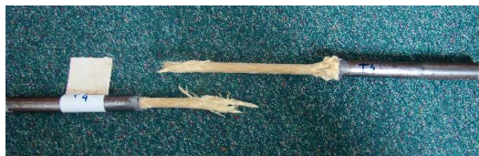
Figure 3: Failure mode after a tensile test.
