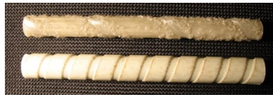
Figure 2: Surface of the GFRP rebars: (top) ASLAN 100, \varnothing 6mm; (bottom) ComBAR, \varnothing 8mm.
