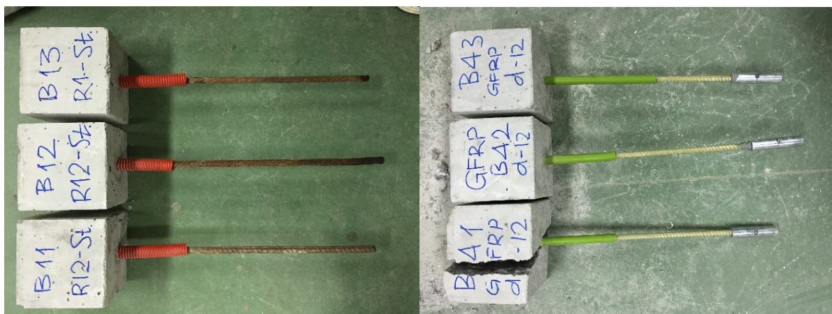
Figure 9 - Specimens for testing of GFRP and Steel rebars – Pull-Out test
