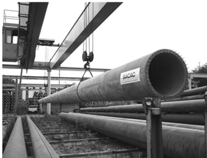
Figure 1: CFRP prestressed pylon made from high performance spun concrete
