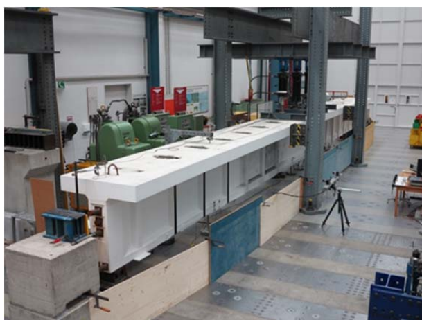
Figure 4: Bridge girder in the Empa laboratory and the force-deflection diagram of the experimental program by Michels et al. [17].
