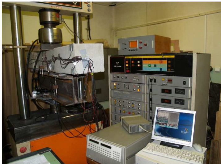
Fig.1 Beam Testing at Instron testing machine
