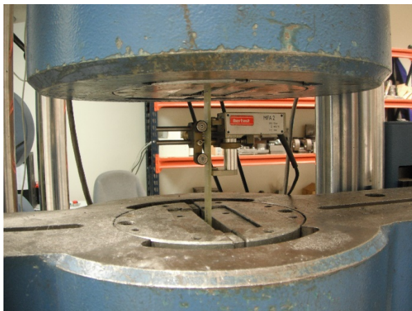
Fig. 2. GFRP tension test according to ISO 527-5.
