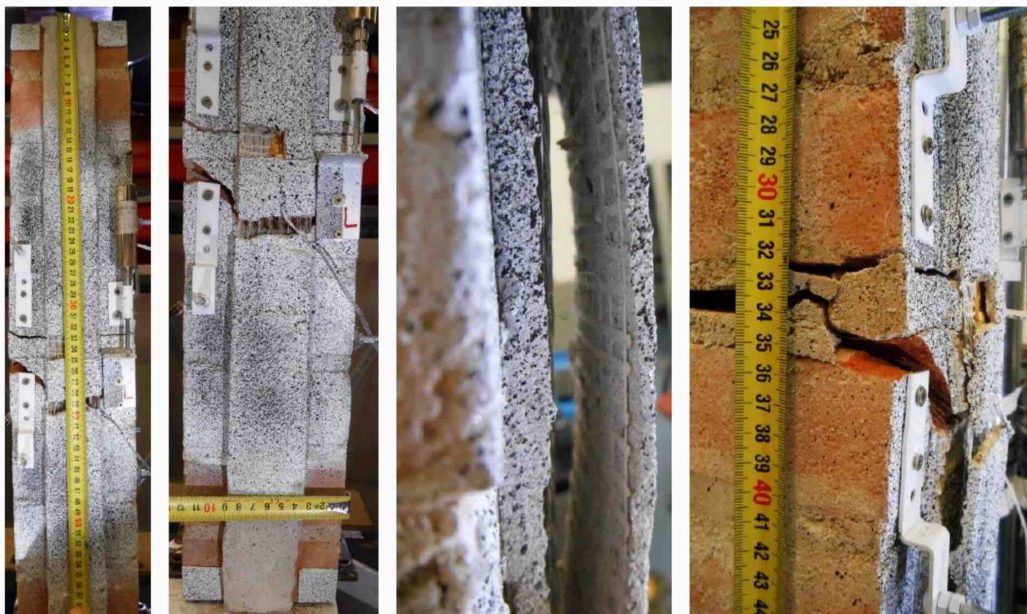
Figure 2. Bond failure between TRM and brick masonry for planar and curved substrates.
