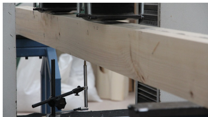
Fig. 5. Four point bending test, according to UNE-EN 408 standard.
