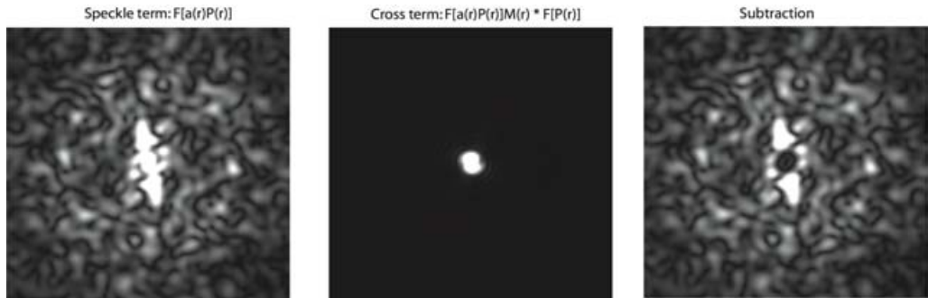
Figure 2. illustration corresponding to Eq.2.6. Left is the speckle term S(\mathbf{r}) = \mathcal{F}[a(\mathbf{r}) P(\mathbf{r})] (modulus). Center: the cross term S(\mathbf{r})M(\mathbf{r}) * \mathcal{F}[P'(\mathbf{r})] . This illustrates that the cross-terms can be neglected outside the mask area. Right: Modulus of the subtraction of the two amplitudes: this shows there is no modification outside the central region corresponding to the mask size.
