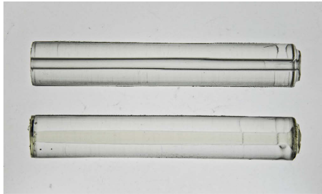
Fig. 2. Preforms: Top, 1185A TPU preform with a 3 mm central hole, bottom, central hole filled with 1185A 10W TPU.
