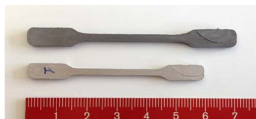
Fig. 2: Green (top) and sintered (bottom) parts.
