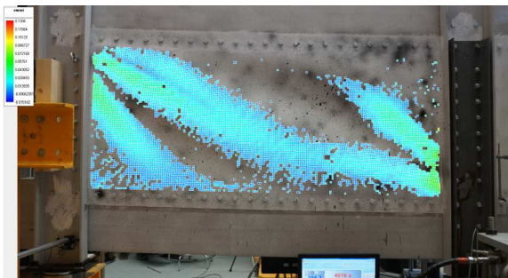
Figure 9. Zones with positive strains in panel during test (DIC visualisation)
