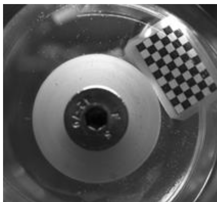
Figure 3. Calibration image with black and white calibration grid
