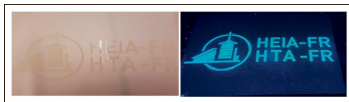
Fig. 5. Our school logo printed by ink-jet with UV curable inks containing CDs. Left: in daylight; right: under UV light (366 nm).
