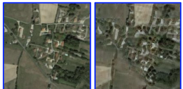
Fig. 2. Sentinel-2 images processed by AI-based 4x upscaling of the uncompressed (left) and JPEG compressed (right) original. While the original images (not shown) appeared identical, the upscaled version of the JPEG image exhibits significant artefacts.
