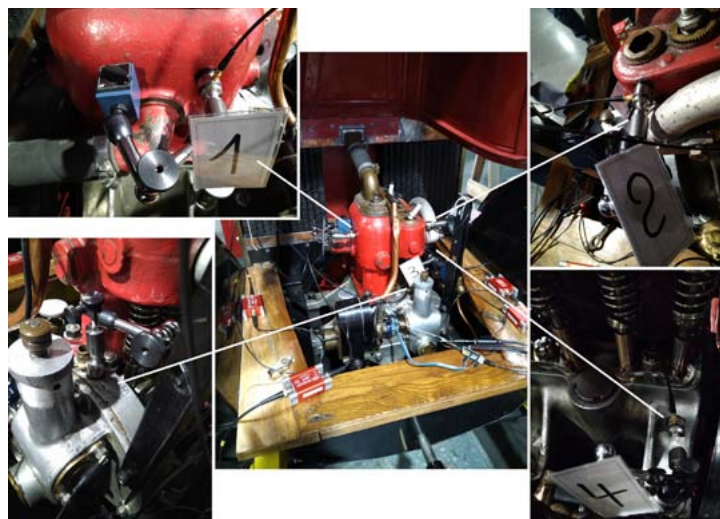
Location of the sensors on the engine ©HE-Arc CR 2019
