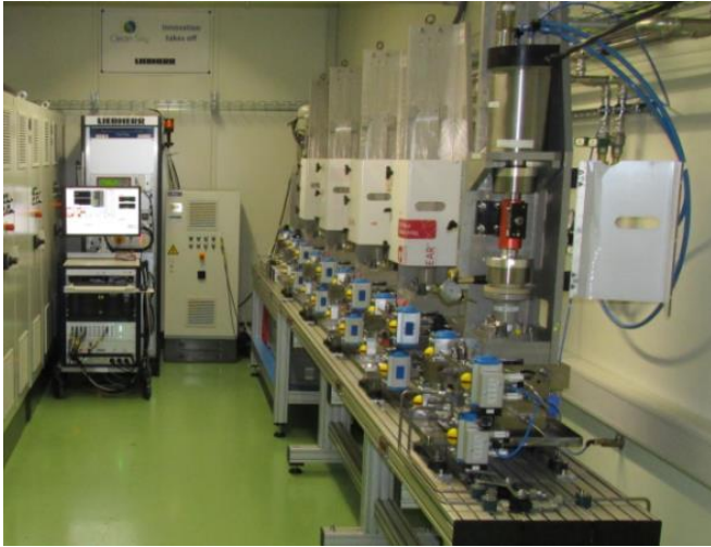
Figure 7: Pump level test rig at Liebherr-Aerospace Lindenberg GmbH
