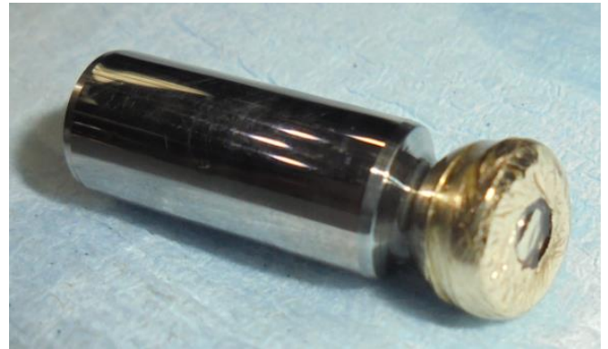
Figure 6: Slipper wear after 35'000 hours of endurance testing
