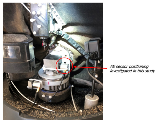
Figure 2. Acoustic emission sensor positioning. As highlighted by the red circle, the AE sensor is glued to the material that is being machined.
