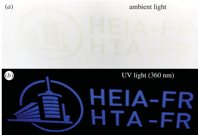
Figure 5. Ink-jet deposition of R-4A dispersed in a UV curable varnish (a) in ambient light and (b) under UV light (360 nm).
