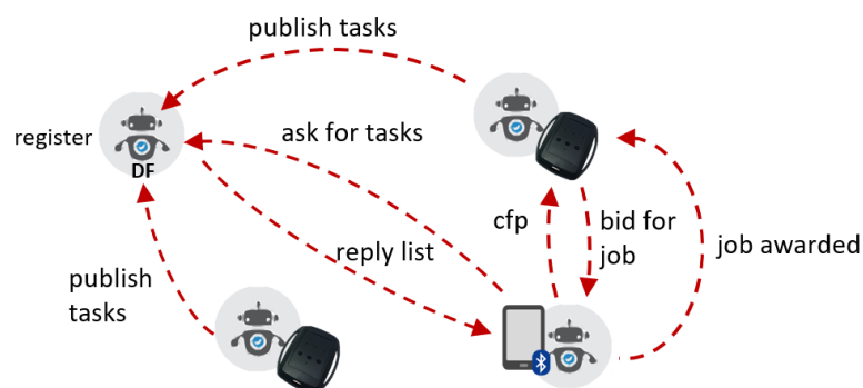
Figure 5. Call-for-proposal interaction among stream processing agents. This interaction can be represented as a FIPA call-for proposals, in which sensor agents publish the tasks they can provide (e.g., sensing and monitoring) in a register agent. Then an application agent can request for agents who are capable of a certain tasks, and emit a cfp. After a bid is performed, the task can be scheduled and executed.
