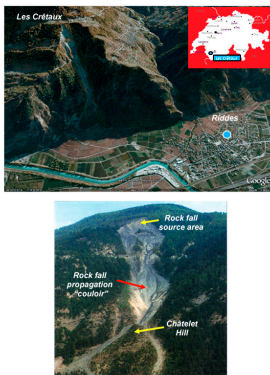
Figure 11. Area of Les Crêtaux, Canton of Valais (Switzerland). Top: location and aerial view of the study site (sources: www.petiteviree.com , Google Earth). Bottom: front view of the rock fall source area and the corridor located just below (source: [17]).
