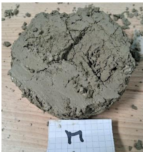
Figure 31: Sample M after thawing.
