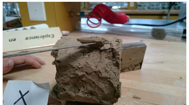
Figure 33: Sample X after thawing (2).
