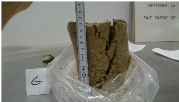
Figure 30: Sample G after thawing (2).
