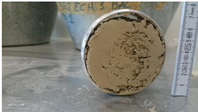
Figure 38: Specimen 3 with voids caused by ice lens.
