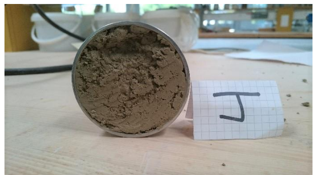
Figure 42: Sample before CRS test 3.
