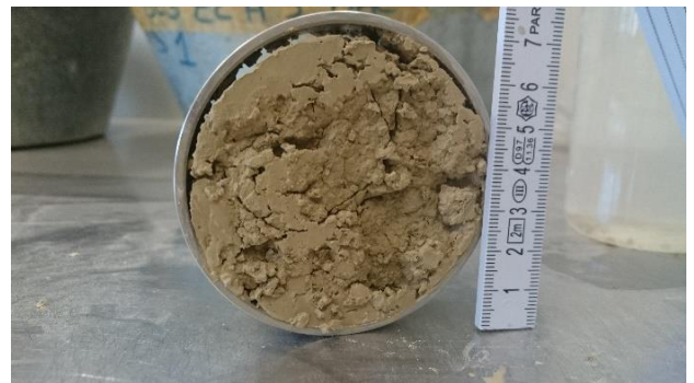
Figure 41: Sample before CRS test 1.
