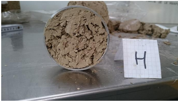
Figure 43: Sample before CRS test 2.
