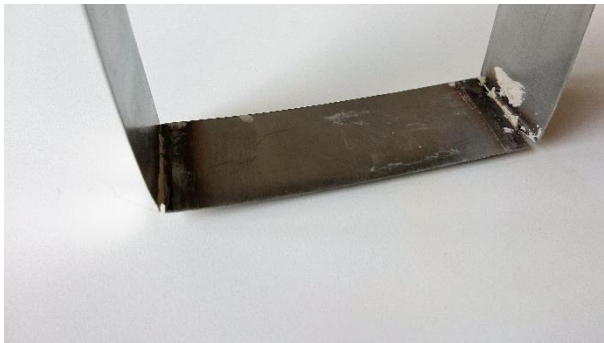
Figure 27: Broken cutting mold (2).
