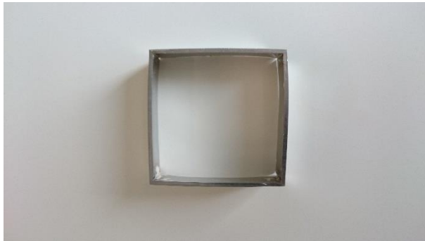
Figure 26: Broken cutting mold (1).
