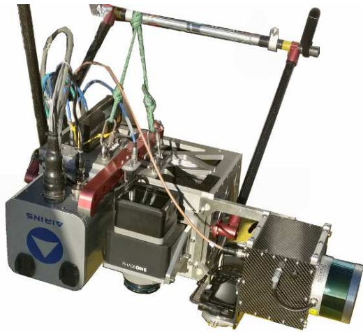
Figure 1: Assembly of 3 IMU's, 2 LiDARs and 2 cameras.
