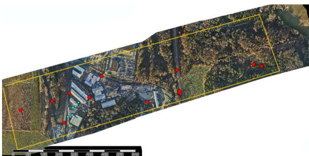
Figure 3: Experimental site near Aclens, Switzerland. Red dots represent GCPs and blue dots the check points.
