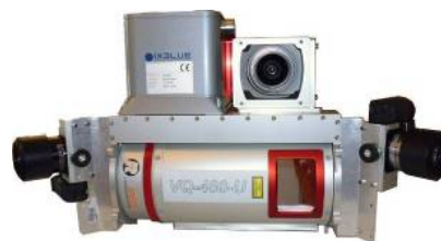
Figure 2: The reference LiDAR sensorhead, mounted with Riegl VQ480U LiDAR.
