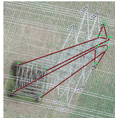
Figure 5: Power tower drawn by hand in Agisoft, similar results can be obtained with other photogrammetric software.
