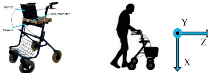
Fig. 1. (a) Hardware setup; (b) Accelerometer axis configuration.
