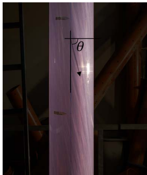
Figure 1. Definition sketch of the control volume of the annular flow (on the left) and photo of a physical model of vertical shaft in operation for an incoming discharge Q = 12.70 \text{ m}^3/\text{s} (Crispino et al. 2016)
