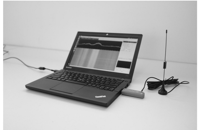
fig.4 Laptop, Realtek RTL2832U, antenna
