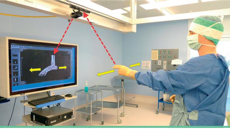
Regarding the depth sensor, we chose to develop our gesture-based interaction system with the Microsoft Kinect sensor 2.0, as its wide field of view allows to track the surgeon inside the sterility area from an outside point of view. Moreover, the Kinect 2, based on time of flight technology (ToF), shows better performance in the high-brightness operating room environment and higher resolution depth data than camera based on structured light technology (e.g. Kinect 1.0) [3].
