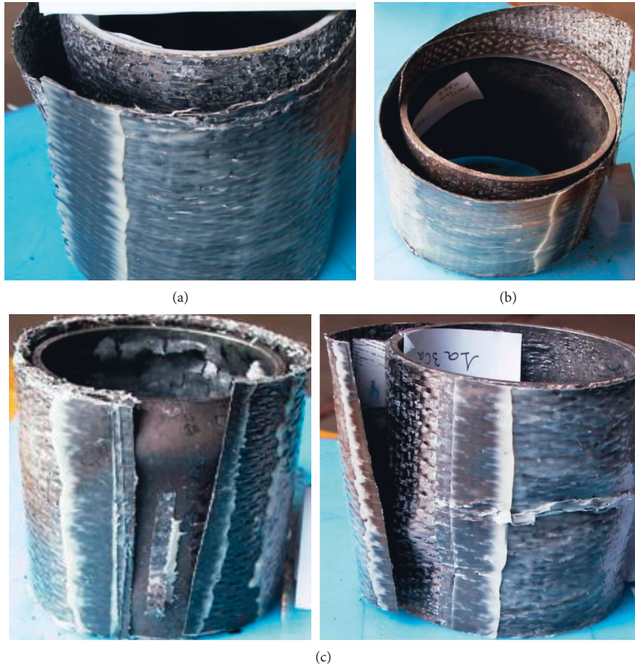
FIGURE 6: (a) Damage to the steel/composite interface; (b) interlayer delamination due to localized loading on CFRP; (c) null or insufficient covering conductors to inhibit “belt effect” of the CFRP layer.
