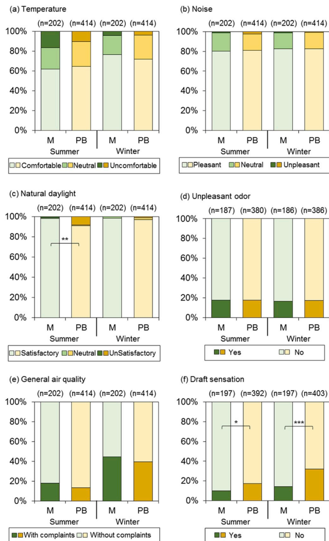
Fig. 6. Comparison of occupants' satisfactions with (a) air temperature, (b) noise, (c) natural daylight, (d) unpleasant odor, (e) general air quality and (f) draft sensation in different seasons between the Minergie-certified (M) and energy-renovated (R) dwellings. * p < 0.05, ** p < 0.01, *** p < 0.001.
