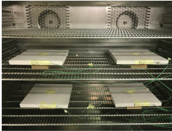
Figure 2: AlbaBalance samples placed in the oven.
