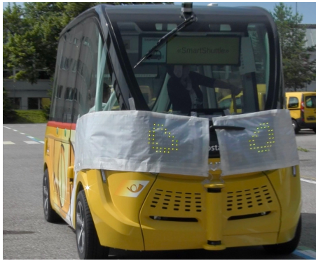
Figure 3: The Intent Communication Interface attached to the driverless shuttle, and displaying the Anthropomorphic signal corresponding to intention “running”.
