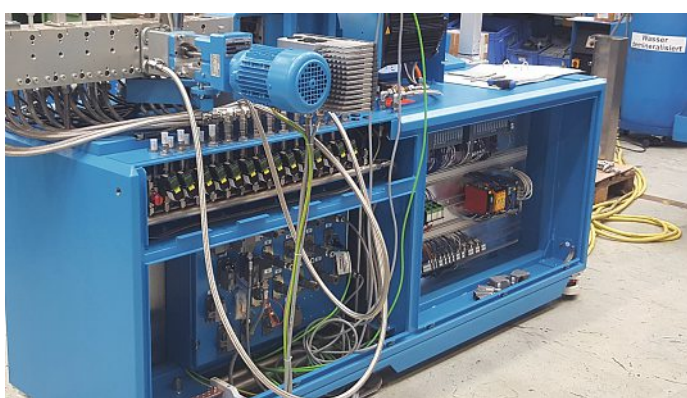
Fig. 4. Twin screw extruder for offcuts reprocessing.
