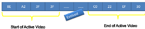
Figure 13. Evolved SAV e and EAV e in Hierarchical level EHW communication protocol
