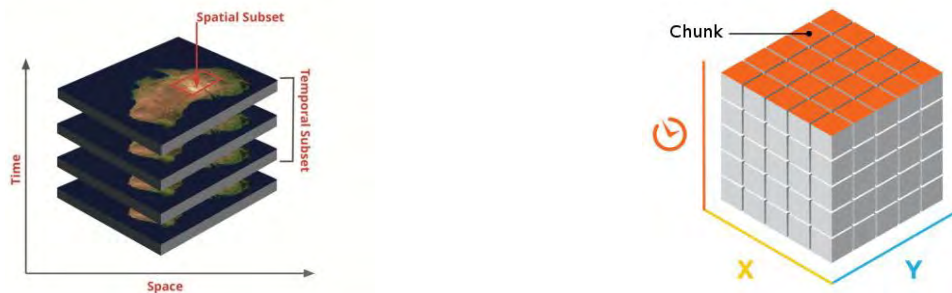
Figure 2. Example of a Rastercube: stacked images on the left and chunks of data on the right
