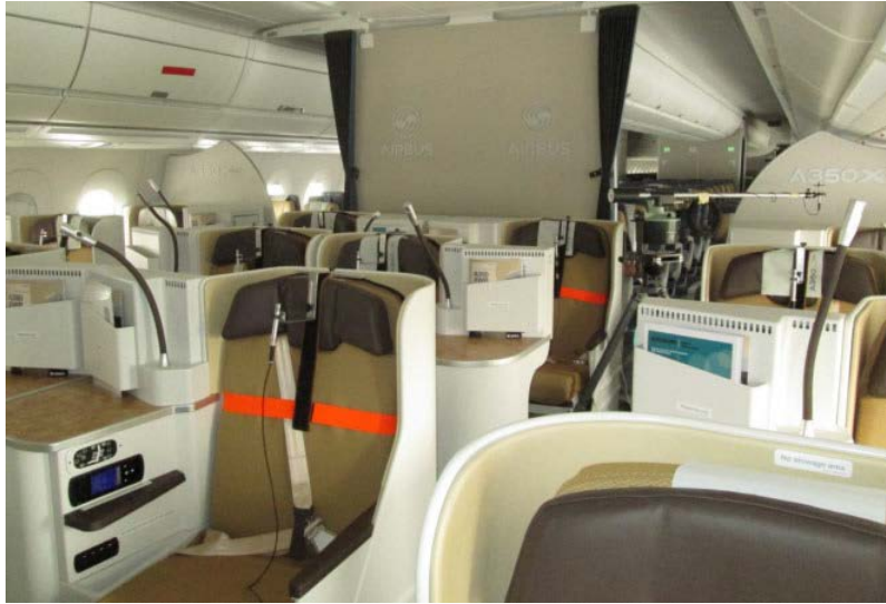
Figure 10: Microphone test setup for sound pressure level measurement within an A350.
