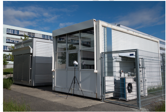
Fig. 21. The embedded photometric device positioned in front of the unilateral façade
