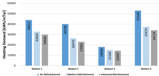
Fig. 4. “Webest” Essen data with refurbishment scenarios.
