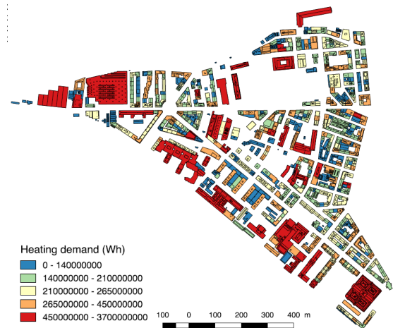
Fig. 7. Space heating consumption of the part of the Jonction district simulated with CitySim under the TMY climate.
