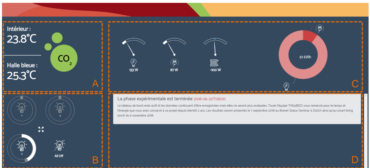
Figure 4 Main menu of the developed interface with comfort indices (A), lighting control (B), instantaneous and proportional electrical consumption (C) and messages window (D).
