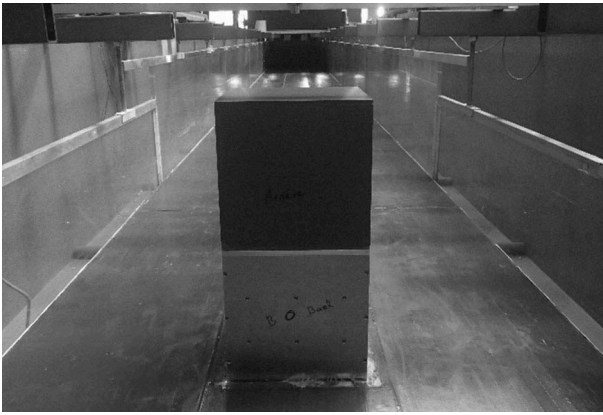
Figure 2. Impervious structural model configuration ( B = 0.3 m, H_B = 0.6 m) used for the present study.
