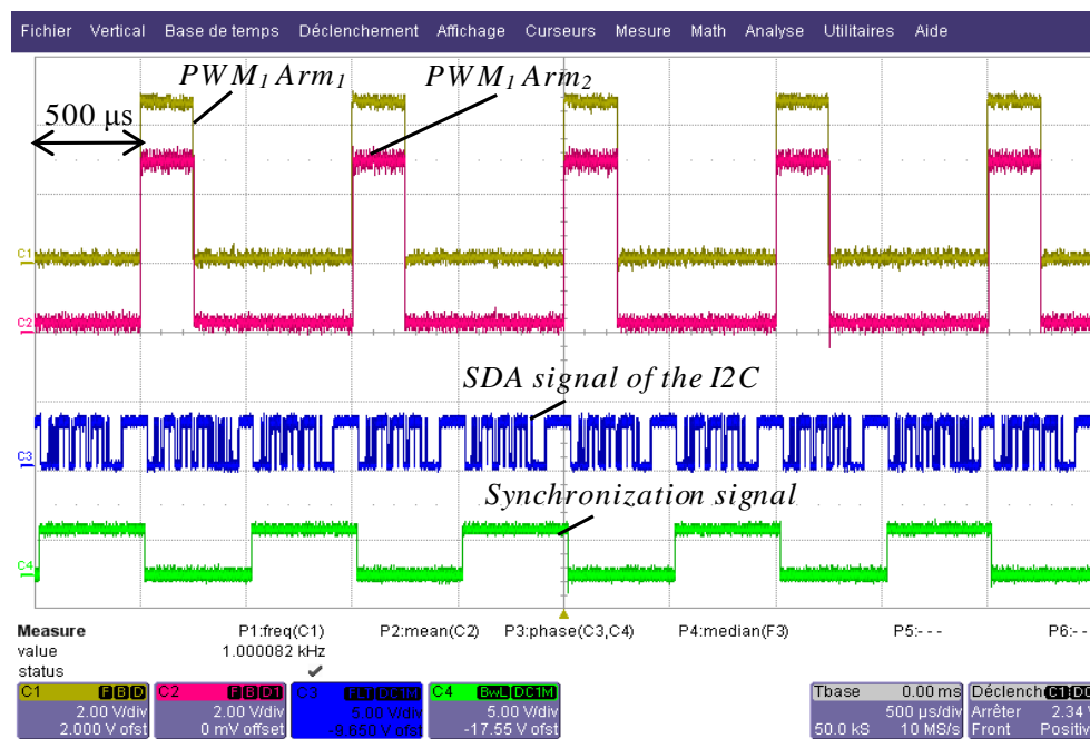
Figure 9. Signals on the converter: PWM 1 signals of two arms controllers (duty cycle 25%), Serial data (SDA) line of the I2C (blue trace) and arms' synchronization signal (green trace).
