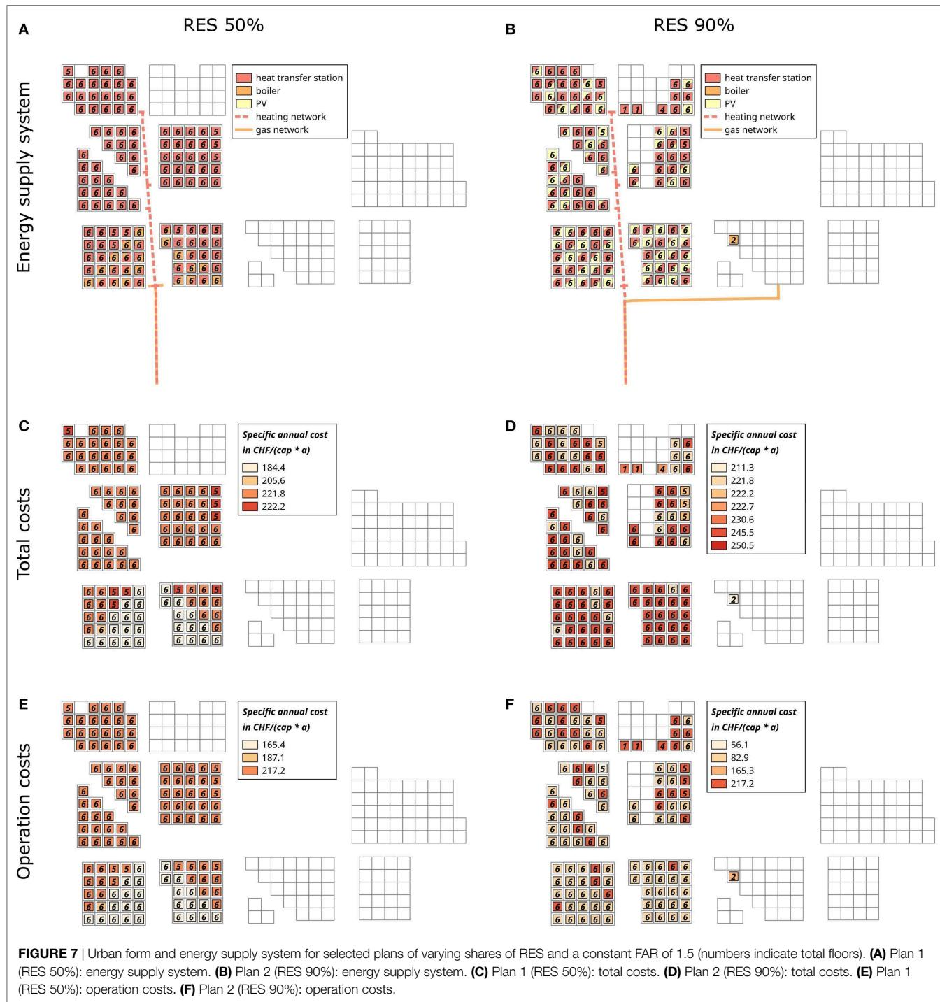
**FIGURE 7 |** Urban form and energy supply system for selected plans of varying shares of RES and a constant FAR of 1.5 (numbers indicate total floors). **(A)** Plan 1 (RES 50%): energy supply system. **(B)** Plan 2 (RES 90%): energy supply system. **(C)** Plan 1 (RES 50%): total costs. **(D)** Plan 2 (RES 90%): total costs. **(E)** Plan 1 (RES 50%): operation costs. **(F)** Plan 2 (RES 90%): operation costs.
