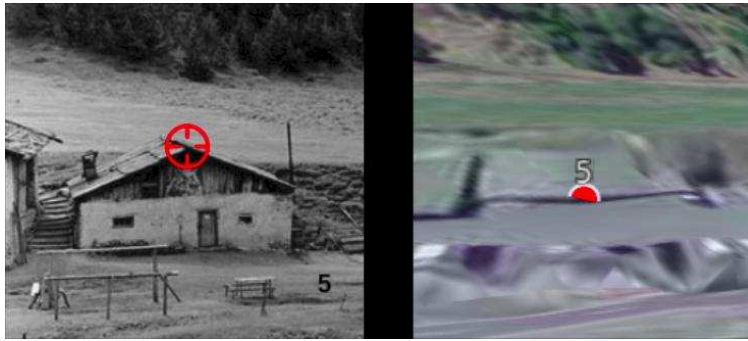
Fig. 5 Incorrect GCP provided on a building. The roof top is clicked in the image, while the same location is provided at ground level in the virtual globe.
