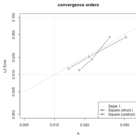
FIG. 6. Perturbation of the identity mapping on the unit square. Convergence of the approximation error \|\mathbf{u}_h - \mathbf{u}\|_{0h} (with structured or unstructured triangulations of the unit square).
