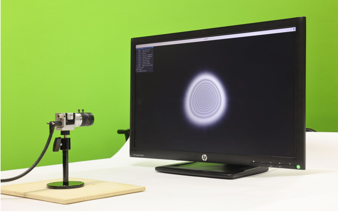
Figure 7. Screen-based experiment setup. The camera is connected to the Jetson via a USB3 cable, fitted with a lens, and positioned in front of a monitor to image the defocused source with known aberrations displayed on the monitor's screen
