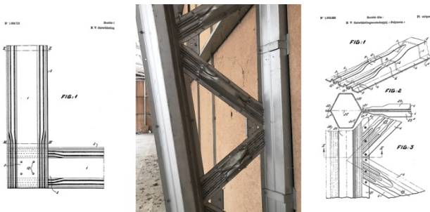
Figure 6. Truss assembly: Patent: R1056719A, published: 02.03.1954 (Jungo). Photo of hall in Fribourg, 2022 (Transform). Patent: FR1078020A, published: 15.11.1954 (Jungo).
