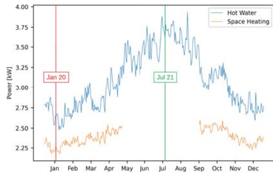
Figure 5: Daily heat pump power for both SH and DHW for a single household. Far from being constant, the SH power ranges from about 2.2 to 2.6 kW whereas the DHW power ranges from about 2.5 to 3.9 kW. There was no detected SH between May and September.
