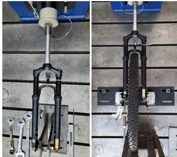
Figure 5. Experimental setups on a dynamical test bench to characterize suspension and tire behavior: the setup with fork suspension alone (left panel) and the setup with both fork and front tire (right panel)
