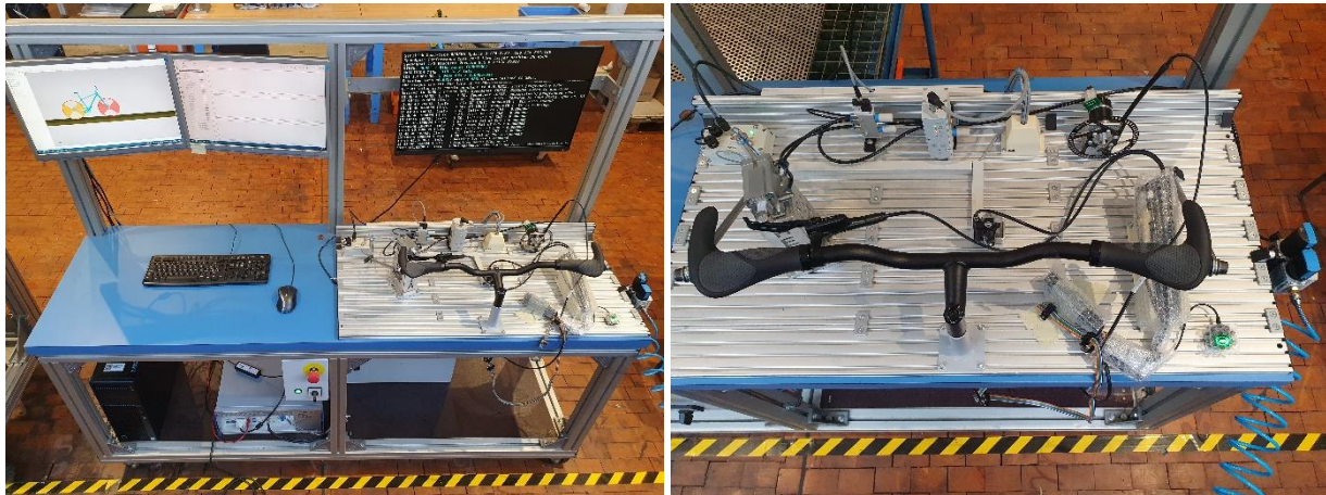
Figure 9. Developed HiL test bench: overview (left panel); handlebar, brake system, and ABS (right panel)
