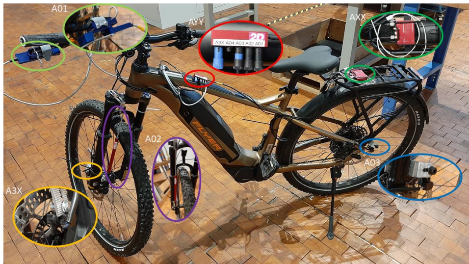
Figure 3. Validation bicycle and equipment (different sensors used are circled)
