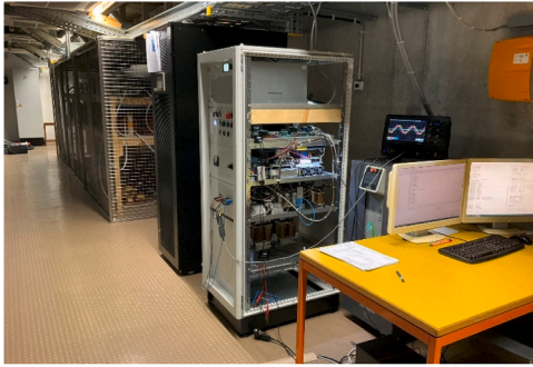
Fig. 18. The 10 kVA prototype inverter in the ReIne laboratory.
