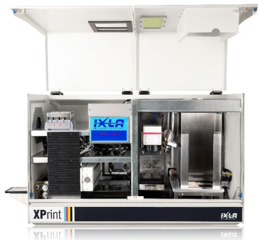
Figure 3 XPrint platform with laser personalisation engine (right) and UV-inkjet engine (left)
