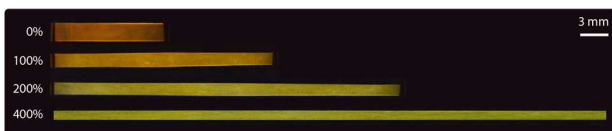
Figure 1: Images taken under UV illumination of an elastomeric polyurethane/tOPV blend film containing 0.2 wt% tOPV subjected to uniaxial tensile deformation at the indicated strains
